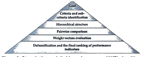
Figure 3: Steps in the analytic hierarchy process (AHP) algorithm.
